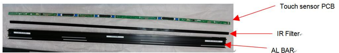
Fig.13 Disassemble AL Bar, IR filter, Touch PCB
