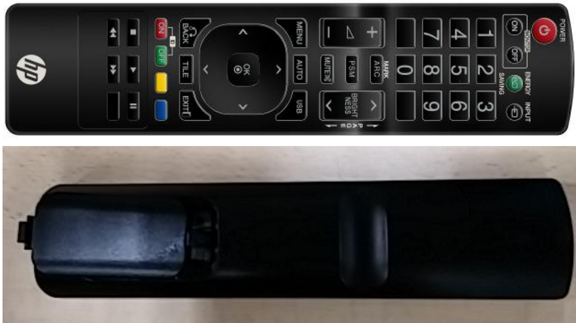
Fig.17 Cover is strongly connected with wire, so it cannot be separated from remote controller
