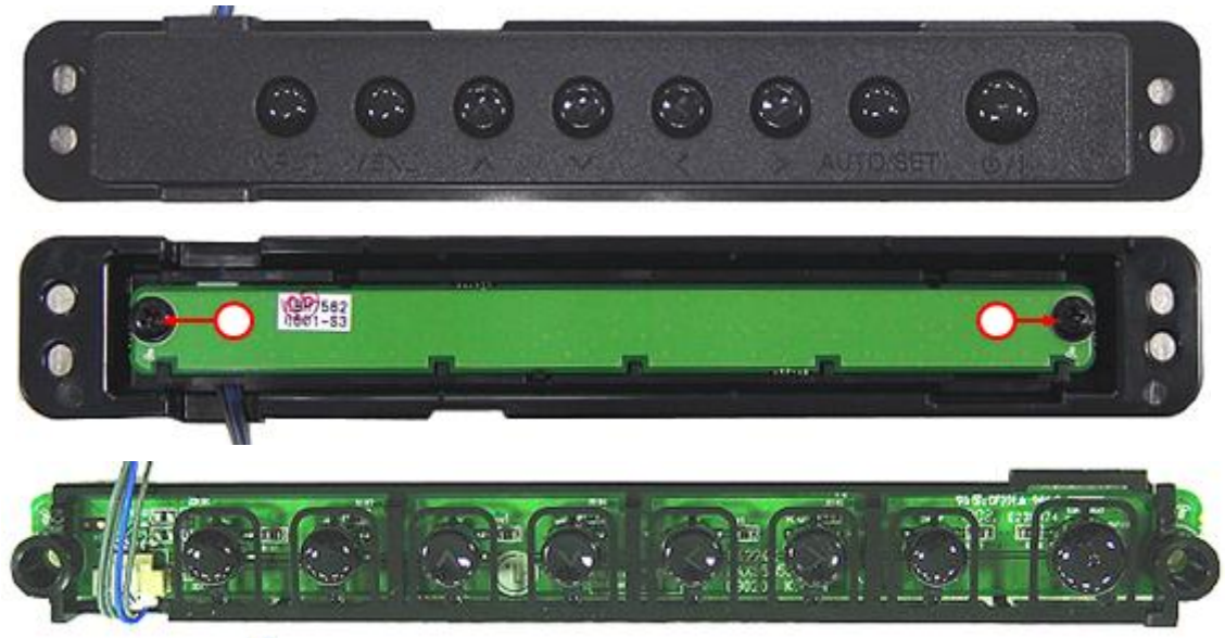
Fig.16 Remove screw 2EA of Control, and Disassemble the control pcb
